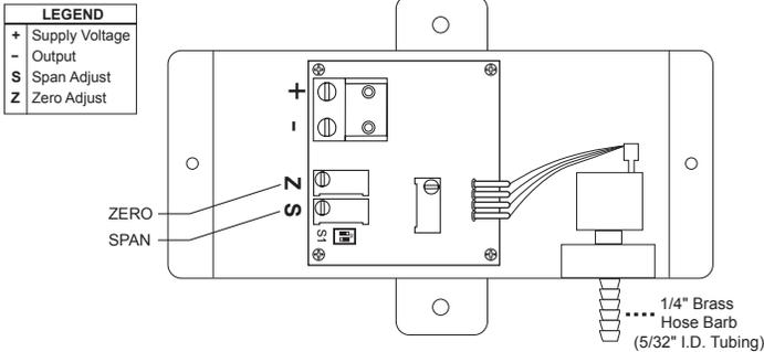
The PR-243 mA output pressure transducers are 4–20 mA output units powered with a 12–40 VDC supply.
