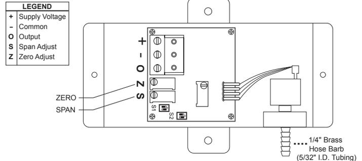
The PR-243 pressure transducers with VDC output are field selectable 0–5 VDC or 0–10 VDC output and can be powered with either a 12–40 VDC or 12–35 VAC.
