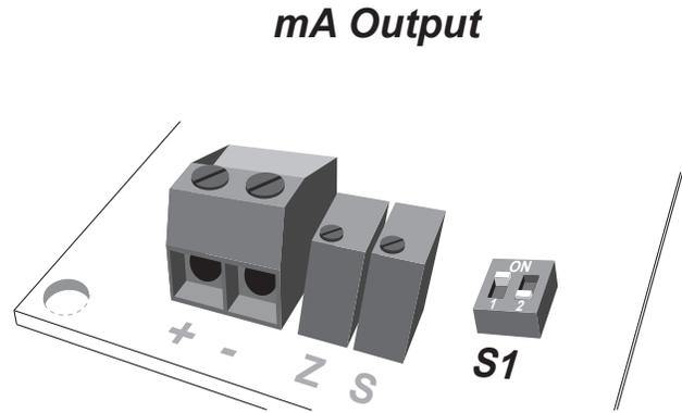
Figure 5 – Range Configurations for Pressure Transducers with mA Outputs
