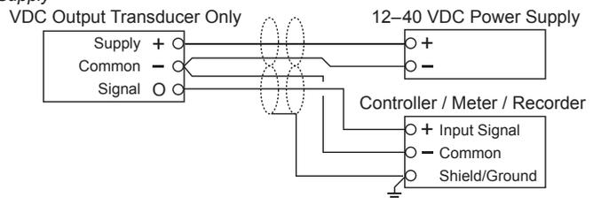
**Caution:** If you are using grounded AC, the hot wire must be on the [+] terminal. Also, if you are using a controller without built-in isolation, use an isolation transformer to supply the PR-243 transducer.
